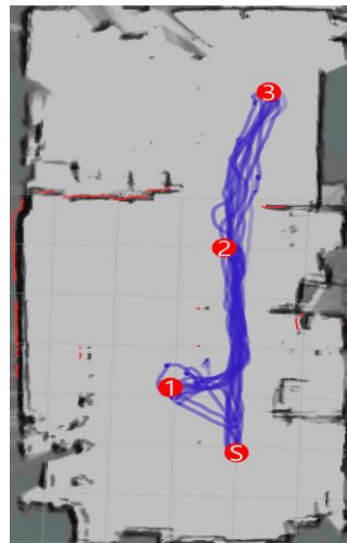
Figure 14. Autonomous navigation result while avoiding 2D and 3D obstacles
